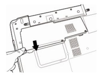
Figure 4-3 Removing the HDD cover
